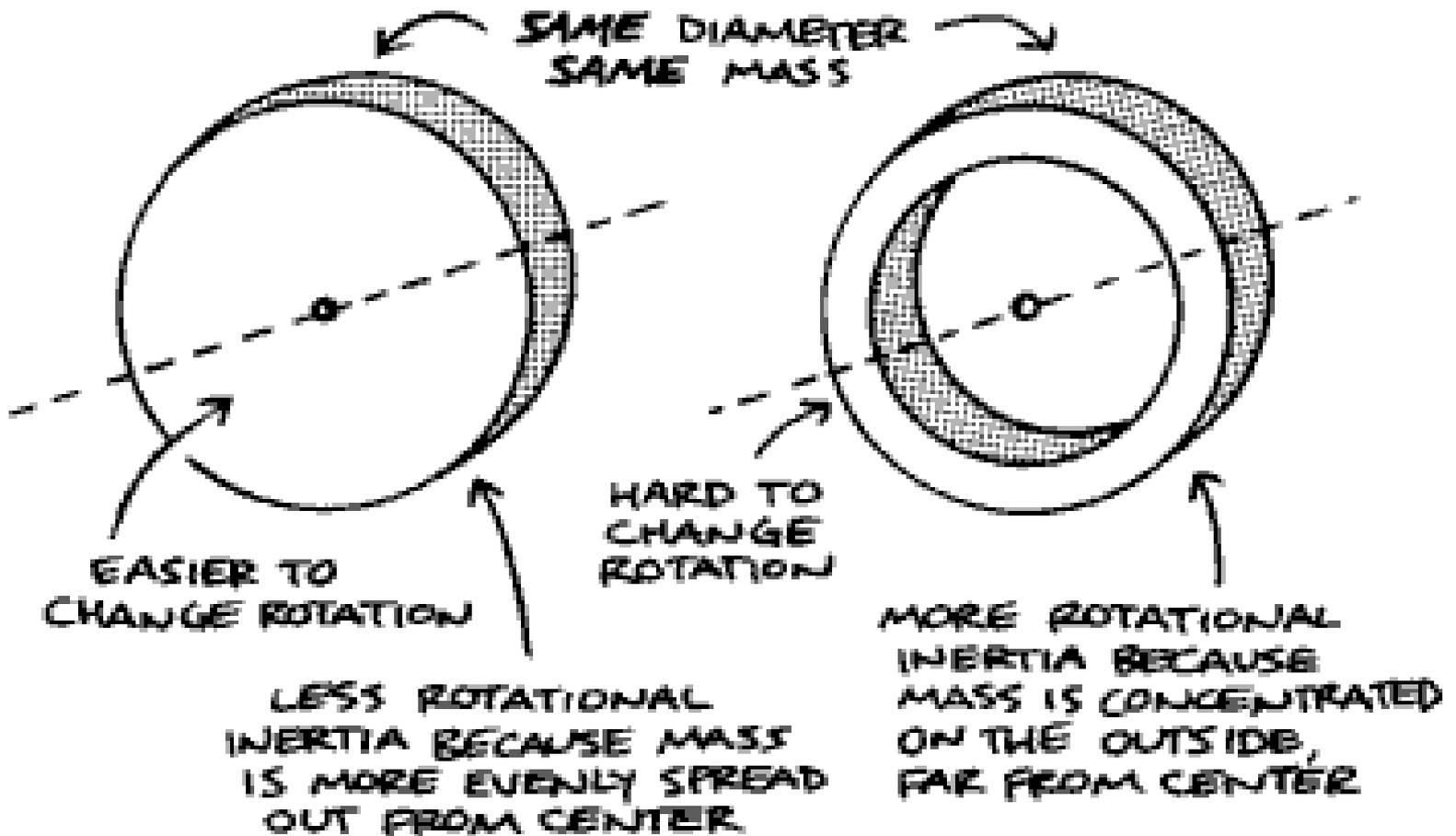
*If two objects have equal mass and radius, the one with more material located far from the center will have a larger moment of inertia*
